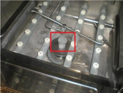
2. ... and press the DRAIN button several times until water is gone.
