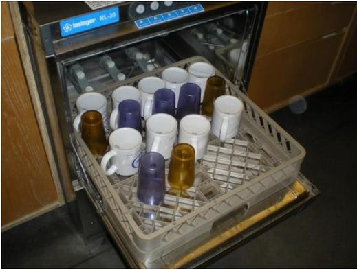
4. Place the loaded rack in the sterilizer, close the door, and press the CYCLE button.
